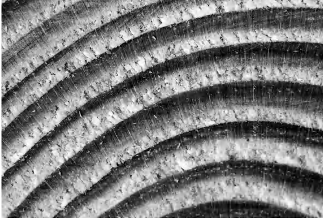
Moisture and a long growing season result in a wide ring, while drought and a short growing season results in a narrow ring.
